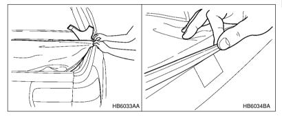
To secure the soft portion of the bed cover to the bed, simply start from either side of the vehicle and place the plastic strip under the rail. Slide your hand down the side of the vehicle pushing the plastic strip under the rail as you go. Continue this around the entire length of the bed. Fasten both closeout wraps with Velcro around the rear chrome bars so that they are secure. Your cover should be tight and ready to conceal items in the bed from view.
