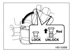
1. Pull the rear seatback locks up and fold down the rear seatback to gain access to the rear quarter pockets at both sides.
