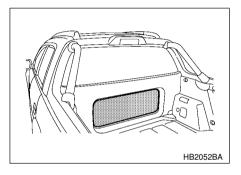
With the switchback door open, you can increase the usable cargo space and can carry long objects.
