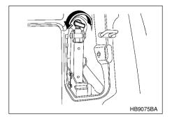
4. Loosen the jack holding screw by turning counterclockwise and remove the jack from the pocket.
