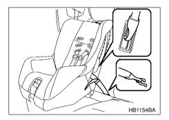
6. While following the instructions supplied by the child restraint system manufacturer, connect the lower hooks onto the lower anchorages located at " are marks on the bottom of the rear seatback. When the hooks are connected, make sure the adjacent seatbelts are not caught.
