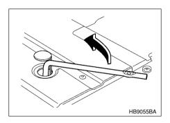
4. Turn the hoist shaft end counterclockwise with the wheel nut wrench until the temporary spare tire is on the ground with enough cable slack to allow you to pull it out from under the vehicle.
