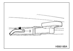
4. Insert the safety pin into the hitch pin securely.
