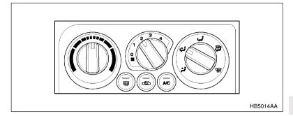
This setting allows you to direct air of different temperatures from the instrument panel and foot outlets. The air from the foot outlets is slightly warmer than from the instrument panel outlets.
