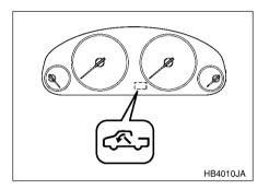
While the ignition switch is in the "ON" position, the switchback door indicator light comes on when the switchback door is open.
