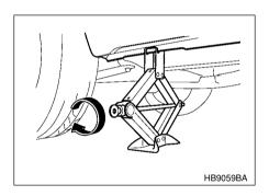
3. Turn the jackscrew by hand until the groove of the jack head engages firmly into the jack-up point.
