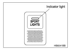
The sport activity lights will operate only when the parking brake is engaged. Push the "SPORT LIGHTS" switch to turn the sport activity lights on.
