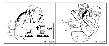
1. Unlock the seatback by pulling the release knob up and then fold the seatback down.
