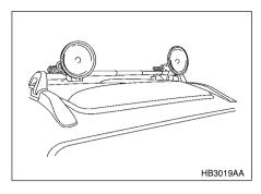
The sport activity lights mount to the vehicle front cross bar. The sport activity lights cross bar wire harness connects to the roof wire harness and then to the vehicle's electrical system.
