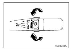
When the wiper switch is in the "\overline{\sqrt{}}" position, turn the dial to adjust the operating interval of the wiper.
