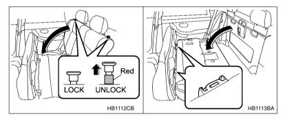
2. Unlock the rear seatback by pulling up on the knob and fold down the rear seatback. Confirm that the pins located at the bottom of the seat cushion is inserted into the slots at the top of the seatback.
