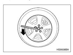
1. Loosen the wheel nuts using the wheel nut wrench but do not remove the nuts.
