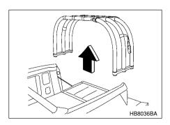
The bed extender can be removed from the vehicle by rotating the extender into a vertical position then lifting straight up.
