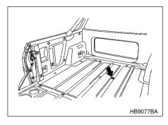
2. Remove the rubber cap from the cargo bed. Store the rubber cap in a safe place. Pay attention not to lose the rubber cap after removal.
