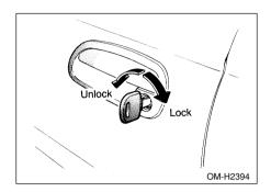
To lock the door from the outside with the key, insert the key into the keyhole and turn the key toward the rear. To unlock the door, turn the key toward the front.
