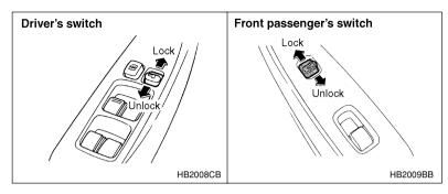
All doors can be locked and unlocked by the power door locking switches located at the driver's side and the front passenger's side doors.
