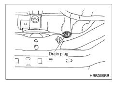
3. Loosen the radiator cap to drain the coolant from the radiator. Then drain the coolant from the reserve tank. Tighten the drain plug securely.
