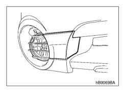
To reinstall the towing hook cover, push it in on both sides while pushing it back to its original position. Make certain that the tabs at the end of the cover are securely inserted into the corresponding slots in the vehicle's body.
