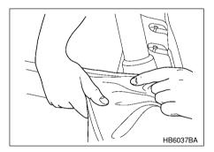
The soft portion of the bed cover can be reinstalled onto the bed cover's hard section. Start by inserting the left front edge of the soft portion into the right side of the hard cover. This area is flared out to ease installation.
