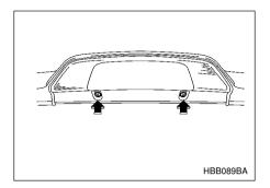
1. Remove the high mount stop light mounting screws.
