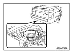
The spare tire is stored in the spare tire holder located under the rear of the cargo bed.
