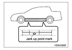
2. Place the jack under the side sill at the front or rear jack-up point closest to the flat tire. Jack-up points are indicated by arrow marks on the side of the side sill skirt.
