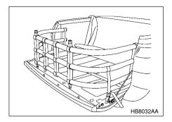
**Open/Outward Position** – To use the bed extender in the open/outward position, simply lower your license plate bracket (see section "Licence plate bracket" under heading of "Tailgate" in Chapter 2), open your tailgate, and rotate the bed extender until it sits on the tailgate.
