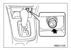
The cigarette lighter operates only when the ignition switch is in "ON" and "ACC" positions.
