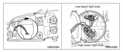
Remove the headlight bulb cover, by turning it counterclockwise.
