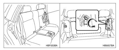
The jack and tool bag are located in the left side rear quarter pocket at the back side of the rear seatback.
