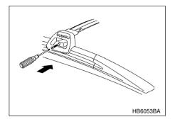
5. Adjust the alignment of the crossbar on the roof rails, and if available, use a T-30 torx® bit and torque wrench and tighten the T-30 torx® head screws to 30 to 35 inch lbs. (3.4 to 4.0 N-m, 0.35 to 0.41 kg-m) of torque (or tighten securely with the torx® wrench provided).
