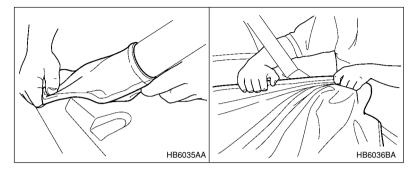
The soft portion of the bed cover can be removed from the bed cover's hard section for cleaning or storage. Unfasten the Velcro on the roll bar closeout wraps and firmly pull the cover out to one side.
