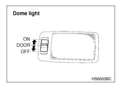
The dome light switch has three positions:
