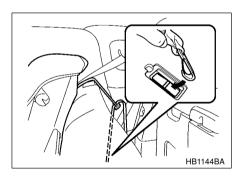
3. Connect the tether belt hook onto the tether anchorage on the backside of the seatback. Take up any slack in the tether belt after connecting it to the tether anchorage.
