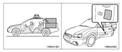
The load capacity of your vehicle is determined by weight, not by available cargo space. The total weight you can carry in your vehicle is shown as the Vehicle Capacity Weight on the tire information label attached to the driver's side door jamb. It includes the total weight of driver and all passengers and their belongings, any optional equipment such as a trailer hitch, roof rack or bike carrier, etc., and the tongue load of a trailer
