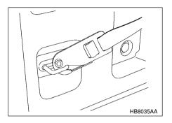
The bed extender should be secured to the rear set of vehicle cargo hooks. Latch the buckle onto the rear cargo hooks and then tighten the tether straps. To disengage the tethers, loosen the tether straps and depress the latch pin.
