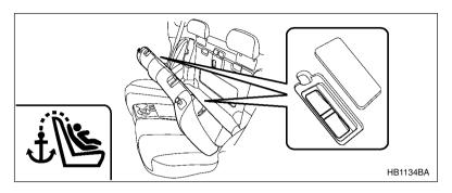
2. Pull the seatback locking knob and fold the seatback forward to see the tether anchorage on the backside of the seatback.
