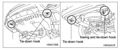
The towing hooks should be used only in an emergency (e.g., to free a stuck vehicle from mud, sand or snow).
