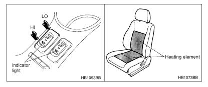
To turn on the seat heater, push the "LO" or "HI" position on the switch, as desired, depending on the temperature. Selecting the "HI" position will make the seat to heat up quickly.
