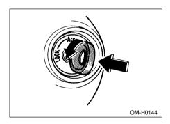
The key can be turned from "ACC" to "LOCK" only when the key is pushed in while turning it.
