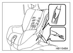
Your vehicle is equipped with four lower anchorages (bars) on the back panel behind the markings on the bottom part of the rear seat-back and two upper anchorages (tether anchorages) on the back side of the seatback for accommodating such child restraint systems.
