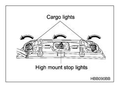
2. Remove the bulb socket from the light assembly by turning it counterclockwise.
