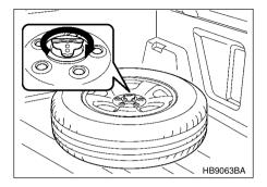
5. Secure the flat tire by tightening the tire holding rod.
