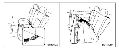
4. Unlock the seatback by pulling the release knob up and fold the seatback down. Confirm that the pin located at the bottom of the seat cushion is inserted into the slot at the top of the seatback.
