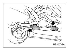
The catalytic converter is installed in the exhaust system. It serves as catalyst to reduce HC, CO and NOx in exhaust gases, thus providing cleaner exhaust.
