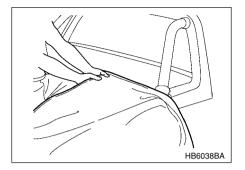
As you insert (and pull) the soft portion of the bed cover into the bed cover's hard section, make sure the next 10 to 15 inches (250 to 380 mm) of the soft portion are straight and ready to enter the flared out portion of the hard section.
