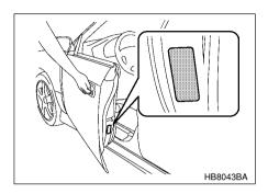
The certification label attached to the driver's side door shows GVWR (Gross Vehicle Weight Rating) and GAWR (Gross Axle Weight Rating). The GVW (Gross Vehicle Weight) must never exceed the GVWR. GVW is the combined total of weight of the vehicle, fuel, driver, all passengers, luggage, any optional equipment and trailer tongue load. Therefore, the GVW changes depending on the situation.
