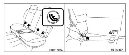
The lower anchorages (bars) are used for installing a child restraint system on the rear seat. For each seating position of the rear seat, two lower anchorages are provided.
