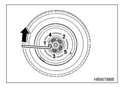
9. Use the wheel nut wrench to securely tighten the wheel nuts to the specified torque, following the tightening order in the illustration.
