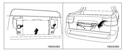
To use the license plate bracket at its lowered/open position, push the two release buttons and pull the license plate bracket up until it clicks. And then open the tailgate.
