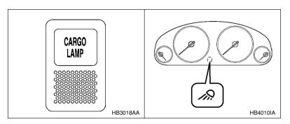
The cargo lamp comes on and goes off whenever the cargo lamp switch is pushed regardless of the position of the ignition switch. The cargo lamp indicator light located in the meter panel will illuminate when the cargo lamp is on.
