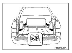
The cargo bed is equipped with four tie-down hooks so that cargo can be secured with a luggage net or ropes.
