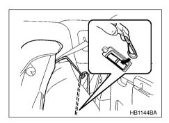
3. Connect the hook of the upper tether belt onto the tether anchorage on the backside of the seatback. Do not allow slack in the tether belt.
