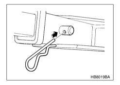
5. Pull the ball mount to make sure it does not come off the hitch receiver
