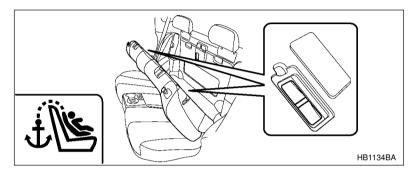
2. Unlock the rear seatback locking knob and fold the seatback forward to see the tether anchorages on the backside of the seatback.
