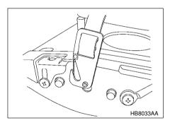
After you have rotated the bed extender, lock the black buckle pin into the tailgate latch by pushing downward until you hear two clicks. Then tighten the tether straps. Repeat this process for the other side. When you want to return the tailgate and the bed extender to the closed/inward position, pull on the tailgate release handle to disengage the tethers.
