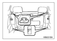
There are four hooks on the back panel behind the rear seatback.
