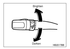
When the lighting switch is in the "506" or " $\equiv D$ " position, you can adjust brightness of the instrument panel illumination for better visibility.
