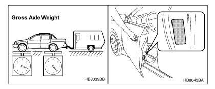
To check both GVWR and GAWR and to confirm that the total weight and weight distribution are within safe driving limits, you should have your vehicle and trailer weighed at a commercial weighing station.
