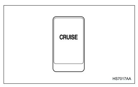
Cruise control enables you to maintain a constant vehicle speed without holding your foot on the accelerator pedal and it is operative when the vehicle speed is 25 mph (40 km/h) or more. Make sure the main switch is turned "OFF" when the cruise control is not in use to avoid unintentionally by setting the cruise control.
