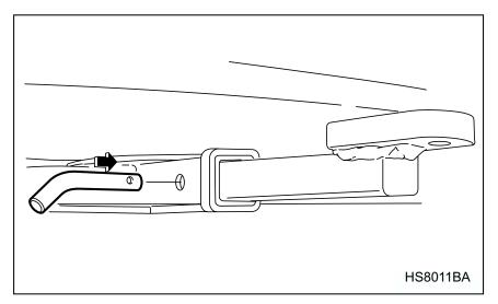
2. Insert the hitch pin into the hole on the hitch receiv-
