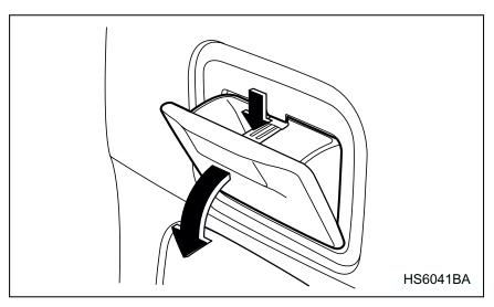
To open the ashtray, pull the upper edge of the lid. Fully close the lid after using it to help reduce residual smoke.
