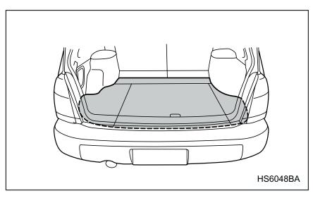
There are four storage trays underneath the floor of the cargo area. They can be used to store small items.
