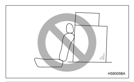
Never stack luggage or other cargo higher than the top of the seatback because it could tumble forward and injure passengers in the event of a sudden stop or accident.
