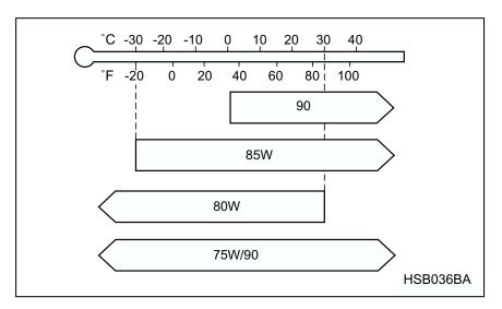
**SAE viscosity No. and Applicable Temperature**
