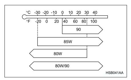
**SAE** viscosity No. and Applicable Temperature
