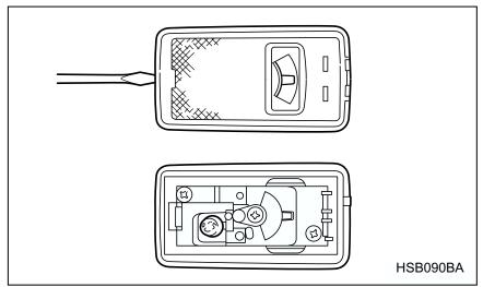
1. Remove the lens by prying the edge of the lens with
