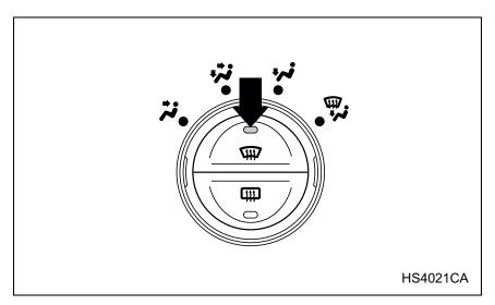
To defrost or dehumidify the windshield and side windows, push the defroster switch " \( \frac{\pmathbb{H}}{\pmathbb{N}} \) ". When the " \( \frac{\pmathbb{H}}{\pmathbb{N}} \) " switch is pushed, regardless whether the air conditioner is operating or not, outside air is drawn into the passenger compartment, the air conditioner compressor turns on, air flow is directed towards the windshield and side windows, and the indicator light on the switch comes on.
