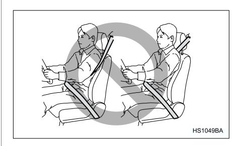
Never place the shoulder belt under the arm or behind the back. If an accident occurs, this can increase the risk or severity of injury.
