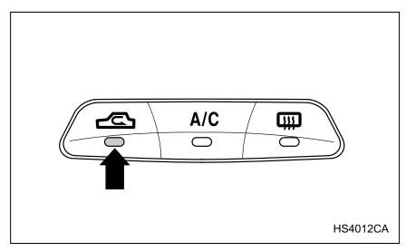
**ON position (Recirculation):** Interior air is recirculated inside the vehicle. Push the air inlet selection button to the ON position. The indicator light will come on.
