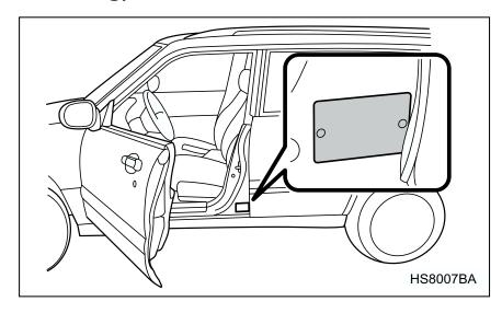
The certification plate attached to the driver's side door jamb shows GVWR (Gross Vehicle Weight Rating) and GAWR (Gross Axle Weight Rating).
