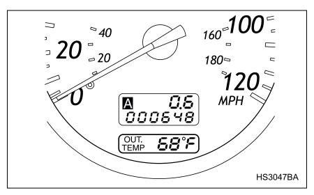
The ambient temperature gauge shows the ambient temperature in a range from –22° F to 122° F (–30° C to 50° C).
