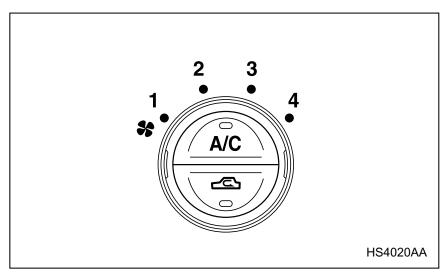
The fan operates only when the ignition switch is in the "ON" position. Select any of the four fan speeds by turning the fan speed control dial. The selected fan speed is indicated by illumination of the corresponding indicator light around the dial.
