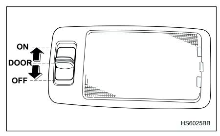
The dome light switch has three positions:
