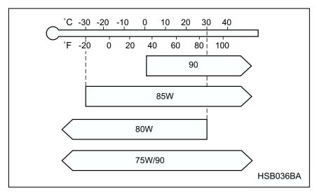
**SAE** viscosity No. and Applicable Temperature
