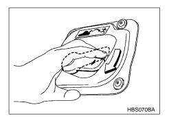
To open the trunk lid from inside the trunk, press the yellow handle downward as indicated by the arrow on the handle. This operation unlocks the trunk lid. Then, push up the lid.
