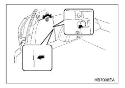
Electrical power (12V DC) from the battery is on tap at the socket when the ignition switch is either in the "ACC" or "ON" position. You can use an in-car use electrical appliance by connecting it to the socket.
