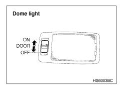
The dome light switch has three positions:
