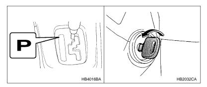
The key can be turned from "ACC" to "LOCK" only when the selector lever is in the "P" position.
