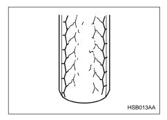
Ride comfort is poor. Also, the tire magnifies the effects of road-surface bumps and dips, possibly resulting in vehicle damage.
