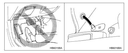
A retaining pin is located on the driver's side of the vehicle next to the fuel filler door release. The floor mat is secured using the built-in grommet, by placing the grommet over the pin and pushing downward.
