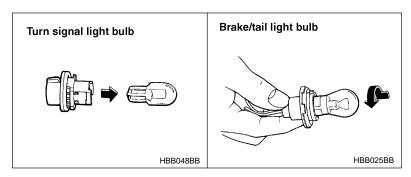
5. Remove the bulb from the socket.
