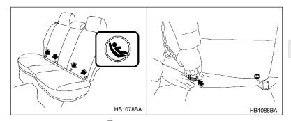
You will find marks " at the bottom of the rear seat seatbacks. These marks indicate the positions of the lower anchorages (bars). Each lower anchorage is located where the seat cushion meets the seatback.
