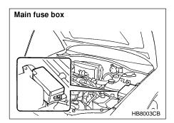
The main fuses are designed to melt during an overload to prevent damage to the wiring harness and electrical equipment. Check the main fuses if any electrical component fails to operate (except the starter motor) and other fuses are good. A melted main fuse must be replaced. Use only replacements with the same specified rating as the melted main fuse. If a main fuse blows after it is replaced, have the electrical system checked by your nearest SUBARU dealer.
