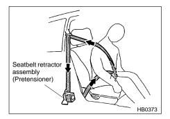
The driver's and front passenger's seatbelts have a seatbelt pretensioner. The seatbelt pretensioners are designed to be activated in the event of an accident involving a moderate to severe frontal collision.
