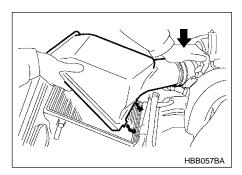
To install the air cleaner case cover, insert the two projections on the air cleaner case cover into the slits on the air cleaner case and then snap the two clamps on the air cleaner case cover.
