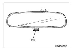
The inside mirror has a day and night position. Pull the tab at the bottom of the mirror toward you for the night position. Push it away for the day position. The night position reduces glare from headlights.
