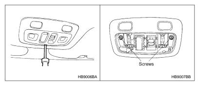
2. Remove the map light lens by prying the edge of the lens with a regular screwdriver, then remove the switch body retaining screws and take off the moonroof switch.
