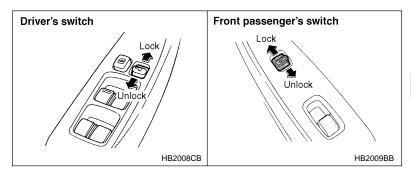
All doors and the rear gate (station wagon) can be locked and unlocked by the power door locking switches located at the driver's side and the front passenger's side doors.
