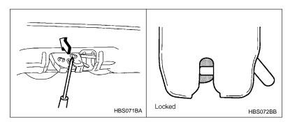
2. Use a screwdriver with a thin blade. Slide the screwdriver blade from the slit aperture of the lock assembly fully to the end until you hear a click. This places the latch in the locked position.
