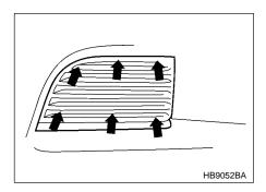
Align the towing hook cover with its original installation position and press all parts of it into place.
