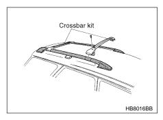
The roof rail is not designed to carry cargo by itself. Cargo can be carried after securing the roof crossbar kit to the roof rail and installing the appropriate carrying attachment. When installing the roof crossbar kit, follow the manufacturer's instructions.
