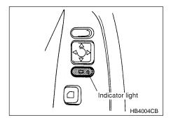
To turn on the outside mirror defogger, push the switch while the engine is running.
