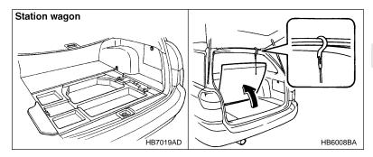
The subfloor storage is located under the floor of the trunk or cargo area and can be used to store small items. To open the lid, pull the tab or handle up.
