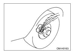
The front disc brakes and the right rear disc brake have an audible wear indicators on the brake pads. If the brake pads wear close to their service limit, the wear indicator makes a very audible scraping noise when the brake pedal is applied.
