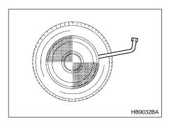
Insert the wheel nut wrench into the notch provided, and pry the wheel cover off.
