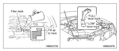
4. Slowly pour the coolant and fill to the radiator filler neck and to the reserve tank's "FULL" level mark. Do not pour the coolant too quickly, as this may lead to insufficient air bleeding and trapped air in the system.
