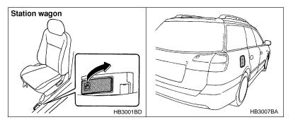
1. To open the fuel filler lid, pull the lid release lever up.
