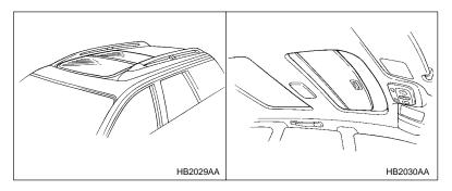
The front moonroof has a tilting function and the rear moonroof has a sliding function.
