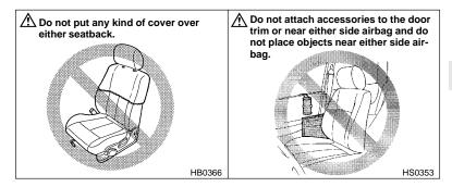
The SRS side airbag is stored in the door side of each front seatback, which bears an "SRS AIRBAG" label.
