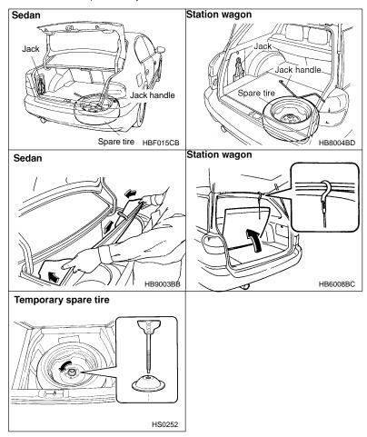
The spare tire is stored under the floor of the trunk or cargo area. To remove the spare tire, proceed as follows:
