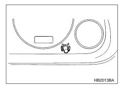
To set the time, turn the setting knob clockwise to advance and counterclockwise to retard the time. 3
