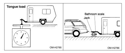
The tongue load can be adjusted by proper distribution of the load in the trailer. Never load the trailer with more weight in the back than in the front; approximately 60 percent of the trailer load should be in the front and approximately 40 percent in the rear. Also, distribute the load as evenly as possible on both the left and right sides.
