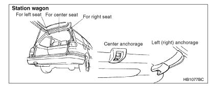
Three anchorages, i.e., ones for the right, center and left positions, are already installed on the rear shelf (on Sedan) or on the rear edge of the roof (on Staion wagon).
