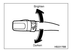
When the lighting switch is in the "₹005" or "≣O" position, you can adjust brightness of the instrument panel illumination for better visibility.
