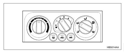
This setting allows you to direct air of different temperatures from the instrument panel and foot outlets. The air from the foot outlets is slightly warmer than from the instrument panel outlets.
