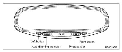
The auto-dimming mirror/compass has an anti-glare feature which automatically reduces glare coming from headlights of vehicles behind you. It also contains a built-in compass.
