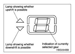
Lamps showing whether upshifting and downshifting are possible: The  $\triangle$  and  $\bigtriangledown$  lamps show whether upshifting and downshifting are possible. When both lamps are off, SPORTSHIFT operation is not possible. When both lamps are on, upshifting and downshifting are both possible. When only the  $\triangle$  lamp is on, only upshifting is possible. When only the  $\bigtriangledown$  lamp is on, only downshifting is possible.
