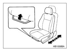
Pull the lever upward and slide the seat to the desired position. Then release the lever and move the seatback and forth to make sure that it is securely locked into place.
