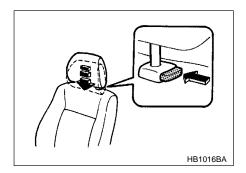
To raise the head restraint, pull it up. To lower it, push the head restraint down while pressing the release button on the top of the seatback.
