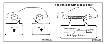
Turn the jackscrew by hand until the jack head engages firmly into the jack-up point.
