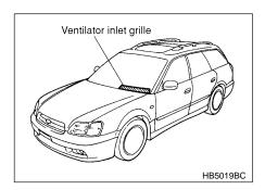
Always keep the front ventilator inlet grille free of snow, leaves, or other obstructions to ensure efficient heating and defrosting. Since the condenser is located in front of the radiator, this area should be kept clean because cooling performance is impaired by any accumulation of insects and leaves on the condenser.
