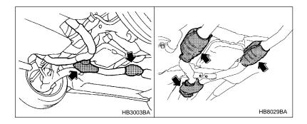
catalyst to reduce HC, CO and NOx in exhaust gases, thus providing cleaner exhaust.
