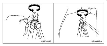
If the jackscrew is too tight to be loosened by hand, loosen it using a screwdriver or the jack handle.
