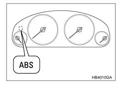
The ABS warning light comes on when the ignition switch is turned to the "ON" position and goes out after about two seconds.
