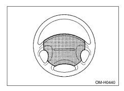
To sound the horn, push the horn pad.
