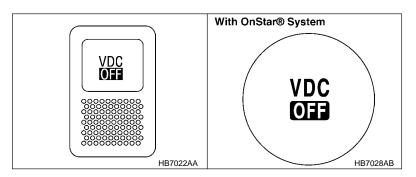
Note: Even when the lighting switch is turned to the "₹0€" or "≣D" position, the "OFF" portion of the symbol stamped on the switch will not illuminate in the dark. Only "VDC" portion will illuminate.
