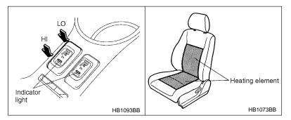
To turn on the seat heater, push the "LO" or "HI" position on the switch. as desired, depending on the temperature. Selecting the "HI" position will cause the seat to heat up quicker.
