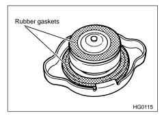
3. After refilling the reserve tank and the radiator, reinstall the caps and check that the rubber gaskets inside the radiator cap are in the proper position.
