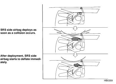
The SRS side airbag can function only when the ignition switch is in the "ON" position.
