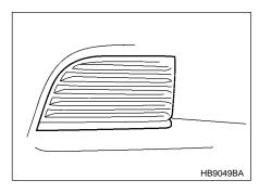
To use the towing hook, insert the top end of the flat tip screwdriver in a slot on the upper part of the cover, and remove the cover while prying it off.
