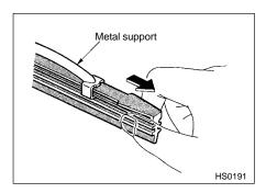
4. If the new blade rubber is not provided with two metal spines, remove the metal spines from the old blade rubber and install them in the new blade rubber.
