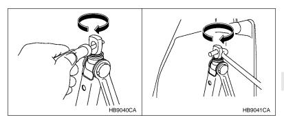
After placing the jack in its storage location, turn the jackscrew clockwise by hand until it becomes too hard to turn. Then, tighten it by an additional 1/4 - 1/3 of a turn using a screwdriver or the jack handle. Unless the jack is properly secured, it may rattle while the vehicle is moving.
