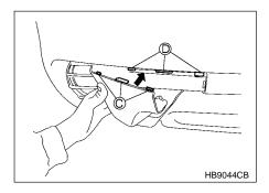
1. Ilnsert the projection  ${\bf C}$  into the hole  ${\bf D}$ .
