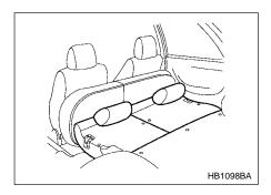
To return the rear seat to its original position, raise the seatback and seat cushion until they lock into place and make sure that they are securely locked.
