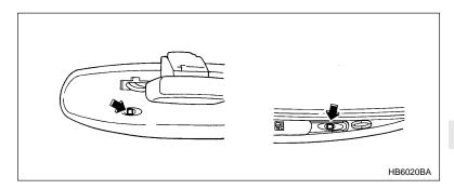
The mirror has a photosensor attached on both the front and back sides. If the glare from the headlights of vehicles behind you strikes the mirror, these sensors detect it and make the reflection surface of the mirror dimmer to help prevent you from being blinded. For this reason, use care not to cover the sensors with stickers, or other similar items. Periodically wipe the sensors clean using a piece of dry soft cotton cloth or an applicator.
