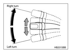
To activate the right turn signal, push the turn signal lever up. To activate the left turn signal, push the turn signal lever down. When the turn is finished, the lever will return automatically. If the lever does not return after cornering, return the lever to the neutral position by hand.
