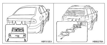
1. Remove the mounting screws using a phillips screwdriver.
