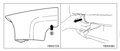
2. Press portion  ${\bf B}$  and simultaneously pull the towing hook cover toward you.
