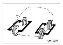
Tire wear varies from wheel to wheel. To maximize the life of each tire and ensure that the tires wear uniformly, it is best to rotate the tires every 7,500 miles (12,500 km). Rotating the tires involves switching the front and rear tires on the right-hand side of the vehicle and similarly switching the front and rear tires on the left-hand side of the vehicle. (Each tire must be kept on its original side of the vehicle.)
