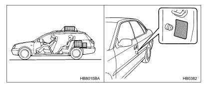
The load capacity of your vehicle is determined by weight, not by available cargo space. The maximum load you can carry in your vehicle is shown as the Vehicle Capacity Weight on the tire information label attached to the driver's side door jamb. It includes the total weight of driver and all passengers and their belongings, any optional equipment such as a trailer hitch, roof rack or bike carrier, etc., and the tongue load of a trailer.
