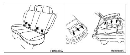
The lower anchorages (bars) are used for installing a child restraint system only on the rear seat window-side seating positions. For each window-side seating position, two lower anchorages are provided. The tether anchorages (upper anchorages) are provided for all the seating positions (middle and both window-side ones) of the rear seat.
