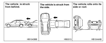
In an accident where the vehicle is impacted more than once, the SRS frontal airbag deploys only once.
