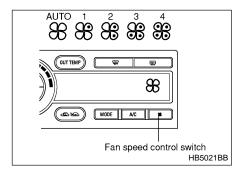
The fan speed control switch has the 5 positions: AUTO position and 4 different fan speed positions.
